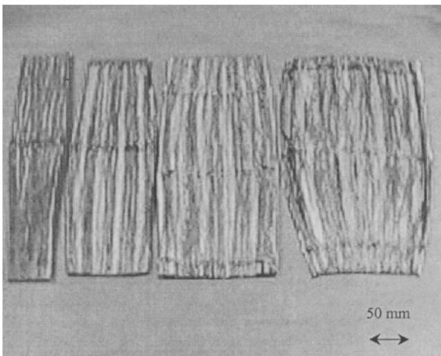
**Fig. 2.** Bamboo zephyr strand mat from Moso bamboo after pre-hot-pressed treatment. From left to right: treatment at temperatures of 100°C, 130°C, 150°C, and 180°C, respectively (Nugroho and Ando 2001; reprinted with permission from the *Journal of Wood Science*)
