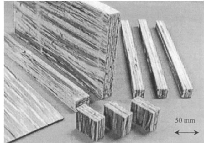
**Fig. 3.** Samples of laminated bamboo lumber (LBL). In the front are specimens of IB (internal bonding) strength. In the background are, from left to right: bamboo zephyr mat, LBL board, and bending testing specimens (Nugroho and Ando 2001; reprinted with permission from the *Journal of Wood Science*)
