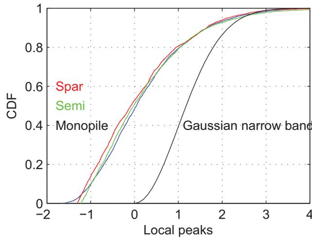
Figure 10. Comparison of a Gaussian narrow-banded process and the distribution functions of the local peaks of the time history of the tower base bending moment  $M(t)$  standardized to zero mean and unit variance for the monopile, spar buoy, and semi-submersible support structures subjected to wind and nonlinear waves
