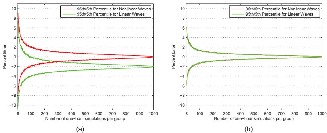
Figure 3. Statistics of the distribution of the percentage error of the mean maximum moment for 1000 random groups for various numbers of one-hour simulations per group, from 6 to 1000. Results are for conditions with wind and linear (green) and nonlinear (red) waves for (a) semi-submersible and (b) spar buoy support structure. In both Figures, error is measured relative to the mean of the maximum moment from the corresponding 1000 simulations under linear waves
