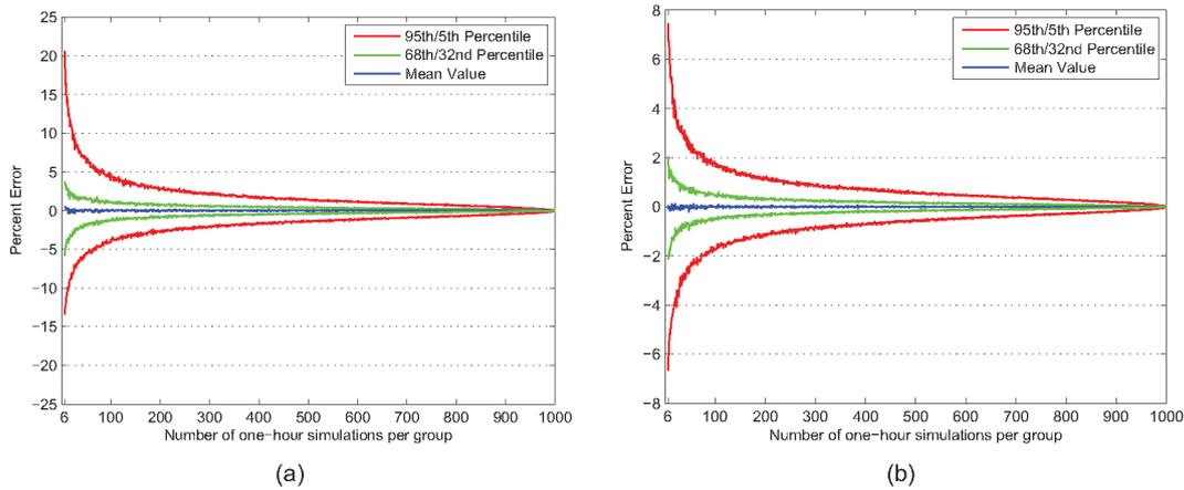
Figure 4. Statistics of the distribution of the percentage error of the mean maximum moment for 1000 random groups for various numbers of one-hour simulations per group, from 6 to 1000. Results are for a monopile support structure under wind and (a) linear waves and (b) nonlinear waves. Error is measured relative to the mean of the maximum moment from all 1000 simulations
