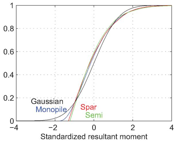
Figure 9. Marginal cumulative distribution functions of the time history of the tower base bending moment  $M(t)$  standardized to zero mean and unit variance for the monopile, spar buoy, and semi-submersible support structures subjected to wind and nonlinear
