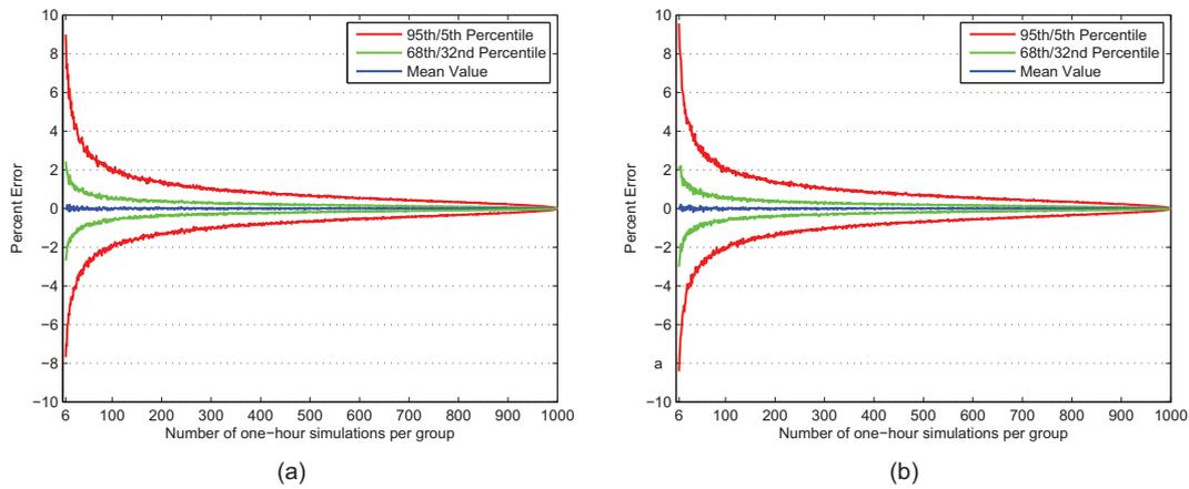
Figure 1. Statistics of the distribution of the percentage error of the mean maximum moment for 1000 random groups for various numbers of one-hour simulations per group, from 6 to 1000. Results are for a semi-submersible support structure under wind and (a) linear waves and (b) nonlinear waves. Error is measured relative to the mean of the maximum moment from all 1000 simulations
