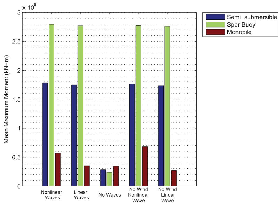
Figure 7. Comparison of the mean of the maximum moment from all 1000 simulations for all three support structures and all five combinations of wind/wave models
