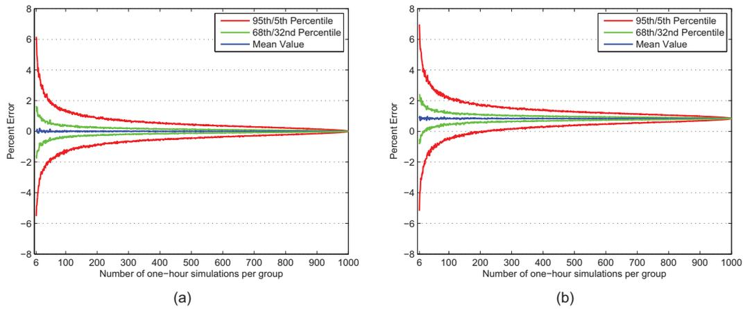
Figure 2. Statistics of the distribution of the percentage error of the mean maximum moment for 1000 random groups for various numbers of one-hour simulations per group, from 6 to 1000. Results are for a spar buoy support structure under wind and (a) linear waves and (b) nonlinear waves. Error is measured relative to the mean of the maximum moment from all 1000 simulations
