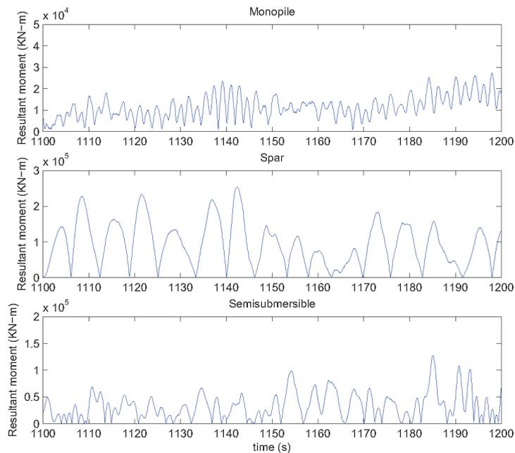
Figure 8. One hundred second samples of the time history of the tower base bending moment  $M(t)$  for the (a) monopile, (b) spar buoy, and (c) semi-submersible support structures subjected to wind and nonlinear waves
