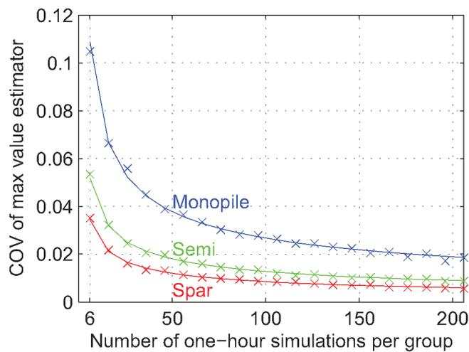
Figure 11. The COV of the estimate of the mean of the maximum moment based on Eq. 3 (solid lines) and results from the simulations with wind and nonlinear waves (x markers) for 500 random groups with various numbers of one-hour simulations per group, from 6 to 200
