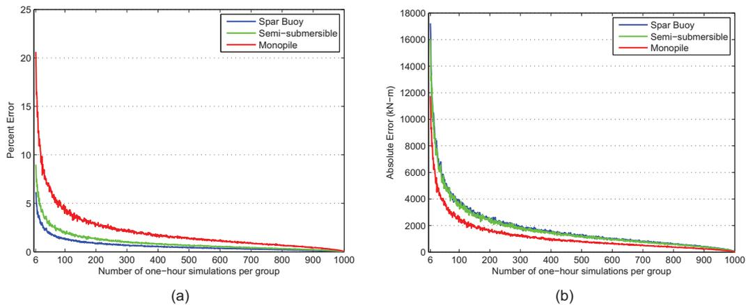
Figure 5. 95<sup>th</sup> percentile values of the distribution of the error of the mean maximum moment for 1000 random groups for various numbers of one-hour simulations per group, from 6 to 1000. Results are for all three support structures and for wind with nonlinear waves. Error is measured relative to the mean of the maximum moment from all 1000 simulations and expressed as (a) a percentage and (b) an absolute value
