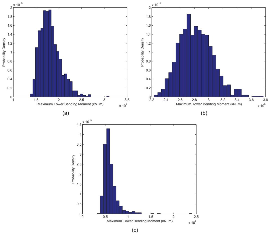
Figure 6. Normalized histograms of maxima from 1000 simulations with wind and nonlinear waves for (a) the semi-submersible, (b) the spar buoy, and (c) the monopile platforms
