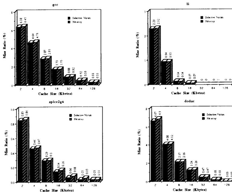
Figure 8: Miss ratio (%) for a selective victim cache configuration with a second-level cache and the hit-array implementation with respect to four **instruction** traces (Line size = 32 bytes, size of victim cache = 8 lines,  $H = 4$ ).
