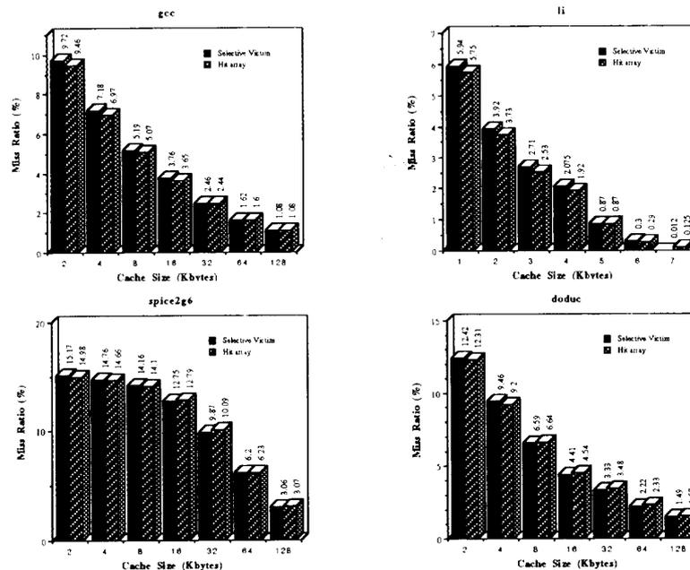
Figure 9: Miss ratio (%) for a selective victim cache configuration with a second-level cache and the hit-array implementation with respect to four **data** traces (Line size = 32 bytes, size of victim cache = 8 lines,  $H = 4$ ).
