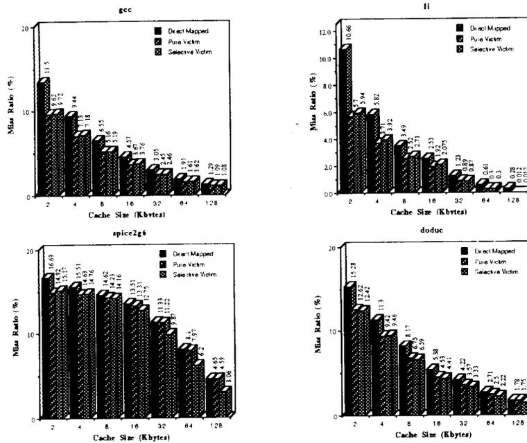
Figure 6: Miss ratio (%) for a direct-mapped cache, a pure victim cache, and a selective victim cache configuration for different cache sizes with respect to four data traces (Line size = 32 bytes, size of victim cache = 8 lines).
