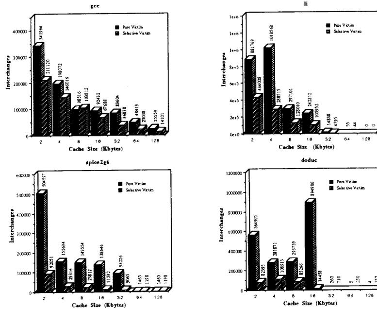
Figure 5: Number of word interchanges for a pure victim cache and a selective victim cache configuration as a function of the cache size with respect to four instruction traces (Line size = 32 bytes, size of victim cache = 8 lines).
