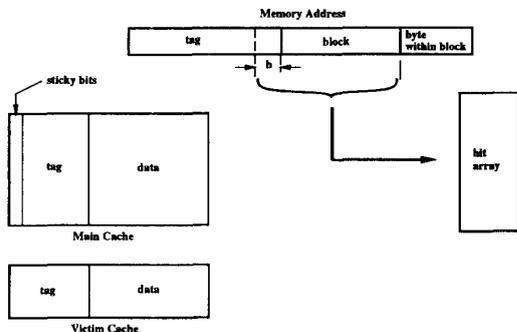
Figure 7: Implementation of the hit-array scheme.
