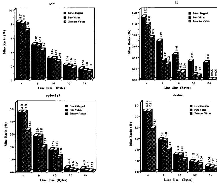
Figure 4: Miss ratio (%) for a direct-mapped instruction cache, a pure victim cache, and a selective victim cache configuration for different line sizes with respect to four instruction traces (Cache size = 16 Kbytes, size of victim cache = 8 lines).
